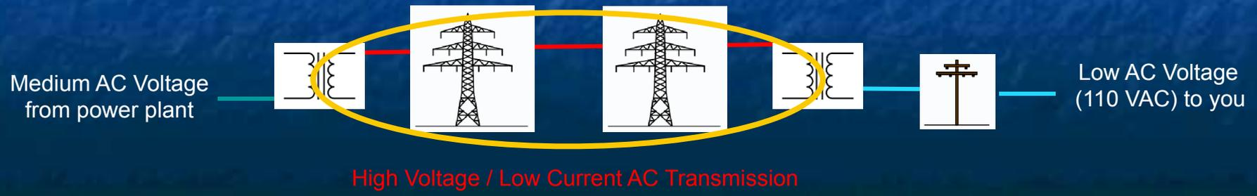
*The transformers are located in "switching yards" or "substations"*
