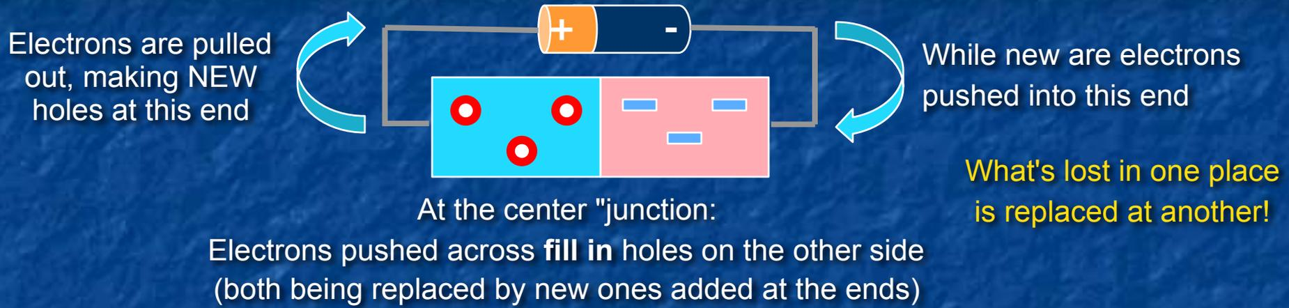
But apply the voltage in other direction and current flow soon grinds to a halt:
