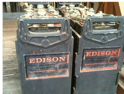
Thomas Edison's nickel-iron batteries used a potassium hydroxide electrolyte manufactured between 1972 and 1975 under the "Exide" brand, originally developed in 1901 by Thomas Edison.
