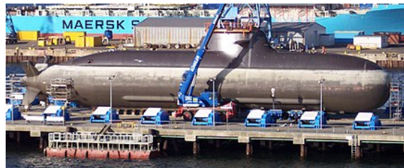
Type 212 submarine with fuel cell propulsion. This example in dry dock is operated by the German Navy.
