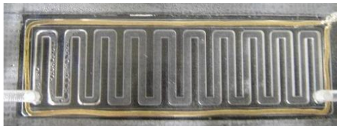
Condensation of water produced by a PEMFC on the air channel wall. The gold wire around the cell ensures the collection of electric current. [24]
