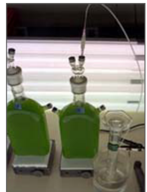
An algae bioreactor for hydrogen production.
