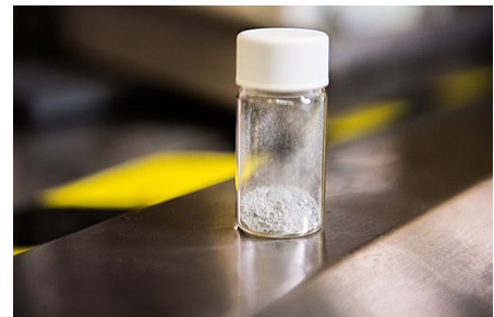
Nano-galvanic aluminum-based powder developed by the U.S. Army Research Laboratory
