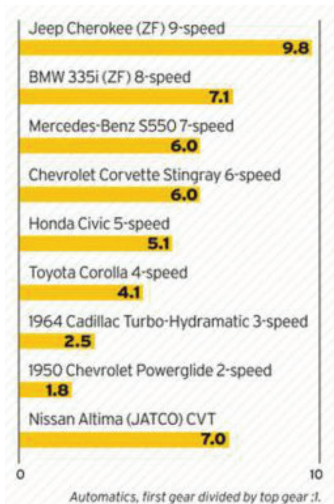
FIGURE 5.13 Increase in ratio spread over the past 65 years. SOURCE: Sherman (2013). Published in Car and Driver magazine, December 2013.
