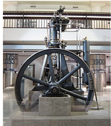
First fully functional diesel engine, designed by Imanuel Lauster, built from scratch, and finished by October 1896. [5][6][7]
