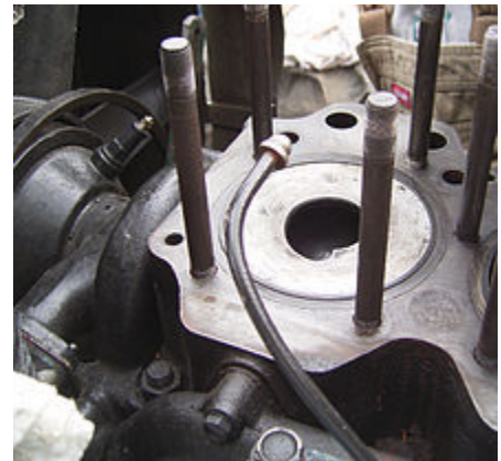
Piston of an MAN M-System centre sphere combustion chamber type diesel engine (4 VD 14,5/12-1 SRW)
