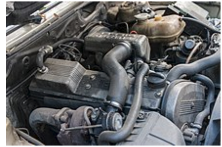
Turbocharged 1980s passenger car diesel engine with wastegate turbocharger and without intercooler (BMW M21)
