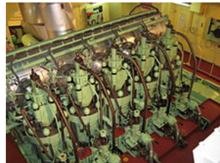
The MAN B&W 5S50MC 5-cylinder, 2-stroke, low-speed marine diesel engine. This particular engine is found aboard a 29,000 tonne chemical carrier.
