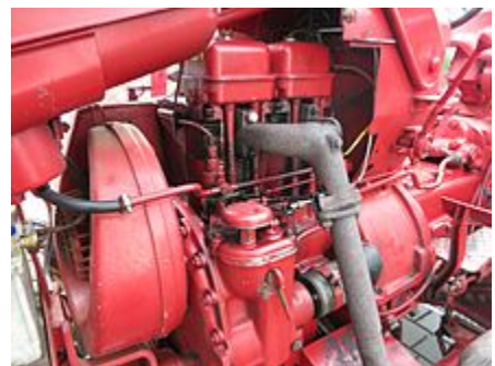
Air-cooled diesel engine of a 1959 Porsche 218
