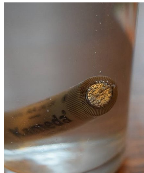
An AA battery in a glass of tap water with salt showing hydrogen produced at the negative terminal
