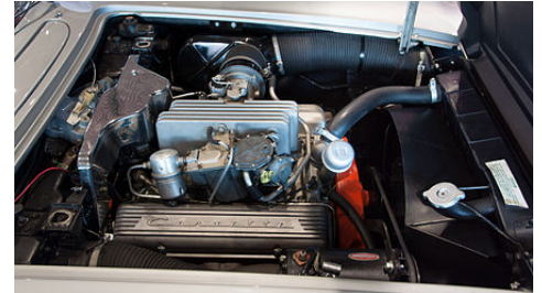
A 1959 Corvette small-block 4.6 litre V8 with Rochester mechanical fuel injection
