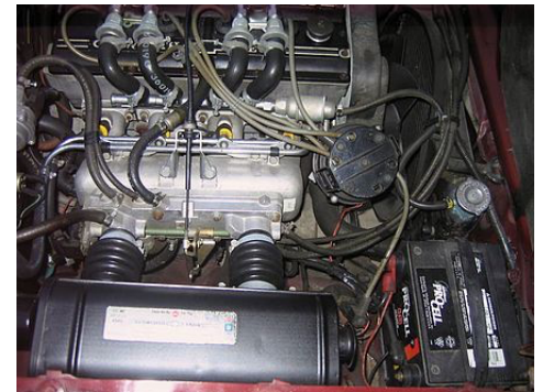
Chevrolet Cosworth Vega engine showing Bendix electronic fuel injection (in orange).
