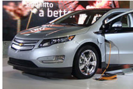
Chevrolet Volt , a plug-in series hybrid , also called an extended range electric vehicle (EREV)
