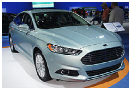
The Ford Fusion Energi is a plug-in hybrid with an all-electric range of 21 mi (34 km).
