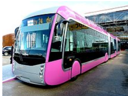
Bus rapid transit of Metz, a diesel-electric hybrid driving system by Van Hool [6]
