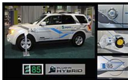
Ford Escape Plug-in Hybrid with a flexible fuel capability to run on E85 (ethanol)
