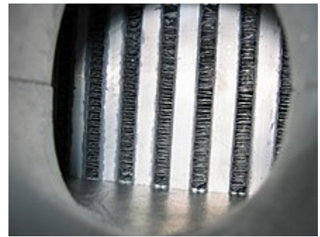
Interior close-up view of an air-to-air intercooler
