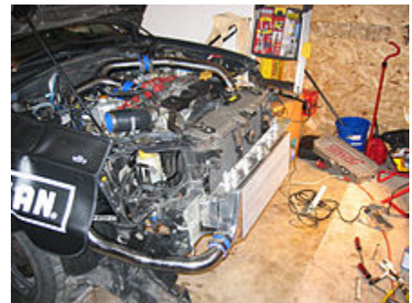
Fitting an after market front-mounted intercooler to a car with a factory-installed top-mounted one
