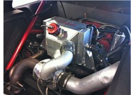
A custom-built air-to-water intercooler, as used in a time attack car
