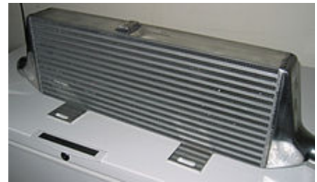
Exterior of the same intercooler core
