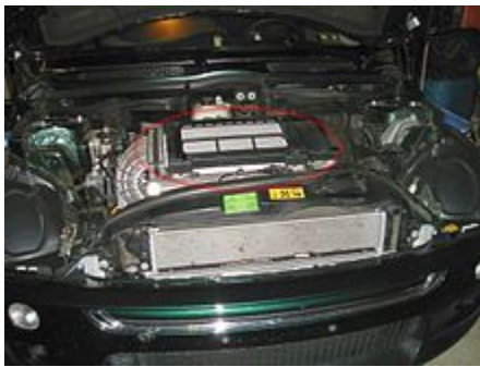
The engine bay of a 2003 MINI Cooper S . The top-mounted intercooler is circled in red.
