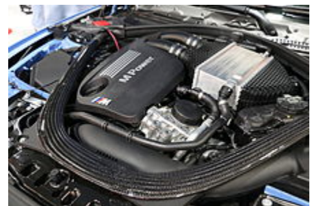
S55 engine in a 2014 BMW M3; the cuboid-shaped metal component is the air-to-liquid charge air cooler.
