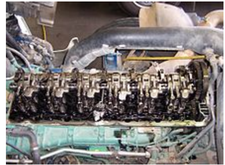
Valve train above a Diesel engine cylinder head. This engine uses rocker arms but no pushrods.
