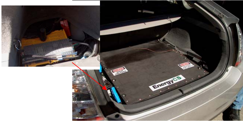
Figure 5-2. Level 1 charger installed on an EnergyCS PHEV Prius.
