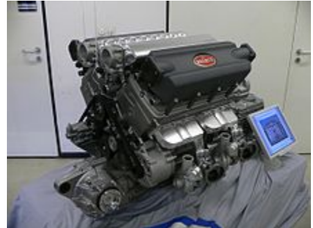
W16 petrol engine of the Bugatti Veyron
