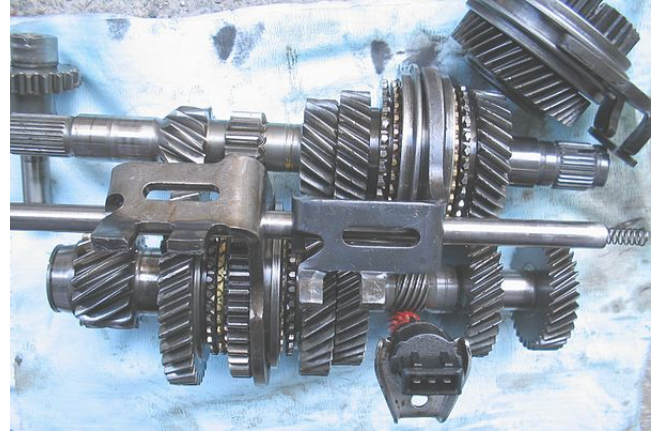
Gears from a five-speed + reverse gearbox from the 1600 Volkswagen Golf (2009).
