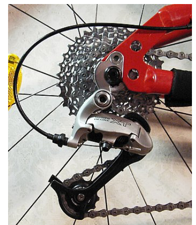
Shimano XT rear derailleur on a mountain bike
