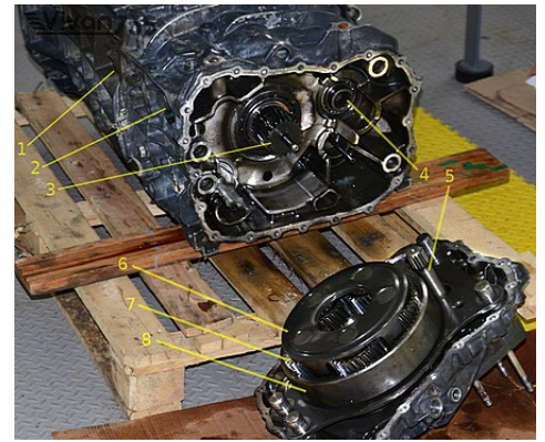
16S181 — opened planetary range housing (2x4x2)
