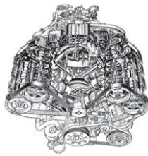
The V6 3.0-liter DOHC/VTEC engine powering Honda's flagship NSX sports car
