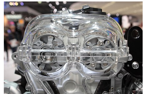
Hydraulic vane-type phasers on a cut-out model of Hyundai T-GDI engine
