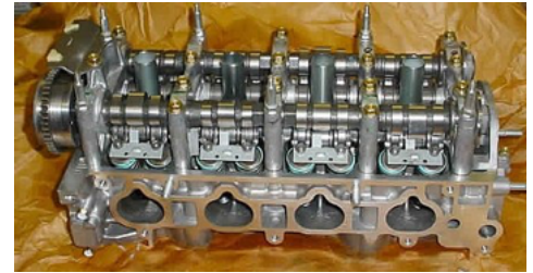
Cylinder head of Honda K20Z3 . This engine uses continuously variable timing for the inlet valves
