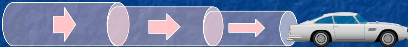
Then, over a time interval  $t$ , the volume of accelerated air =  $A_{\text{air}} \times (v_{\text{steady}} \times t)$
