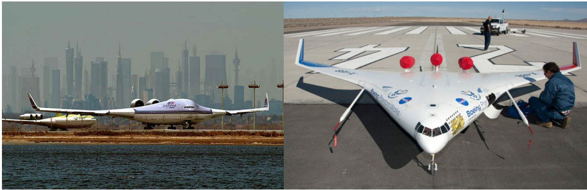
Figure 2: The Blended Wing Body operational concept (left) and Boeing X48C BWB prototype (right) (Vicroy, 2011)
