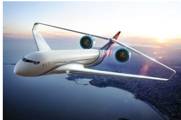
Figure 4: The Box Wing Aircraft concept – left ("Boxplane wing and aircraft," 1974) & Box Wing Airliner - right (Picture by Nick Kaloterakis)
