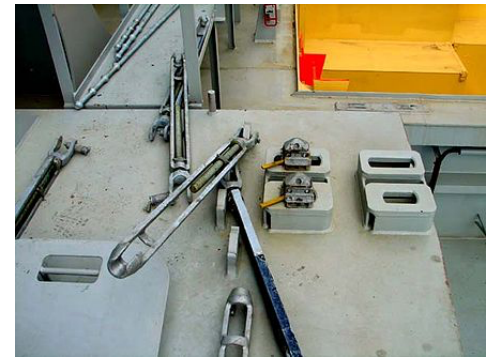
Twist-locks and lashing rods (pictured) are widely used to secure containers aboard ships.
