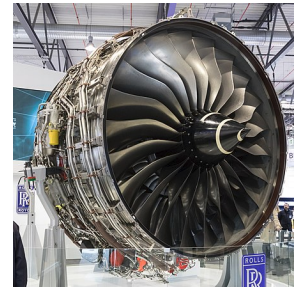
The 3.00 m (118 in) fan of the Trent XWB
