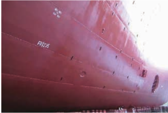
Figure 23. OLIVIA MAERSK Showing Wing Air Induction Pipe Micro-bubble Units Staggered Over its Side
