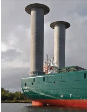
Figure 26. Flettner Rotors on ENERCON E-Ship 1
