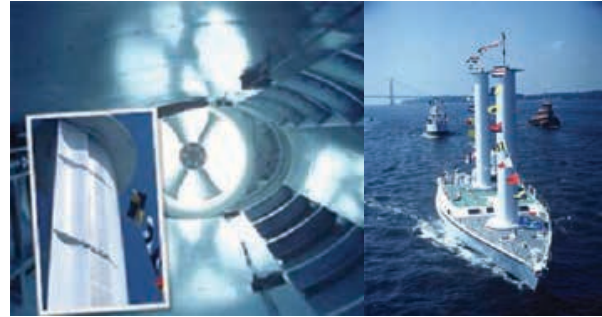
Figure 28. Turbosails on the ALCYONE
