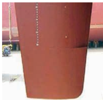
Figure 12. Twisted Leading Hedge Rudder on the CMA-CGM Containership CHRISTOPHE COLOMB
