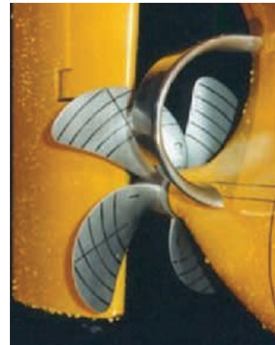
Figure 8. Model of a Schneekluth Duct
