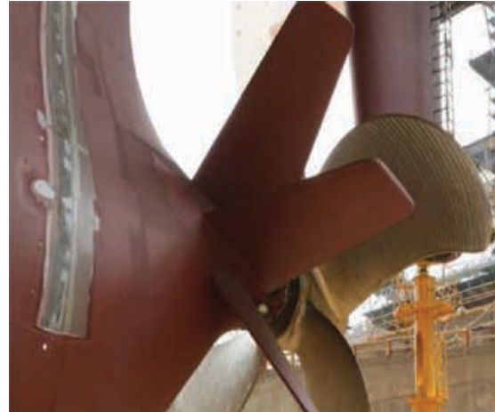
Figure 10. Stators on CMA-CGM Containership CHRISTOPHE COLOMB
