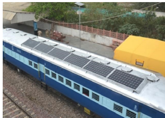
Figure 3: A train coach fitted with solar panels in India. Source: Financial Express, (2016).
