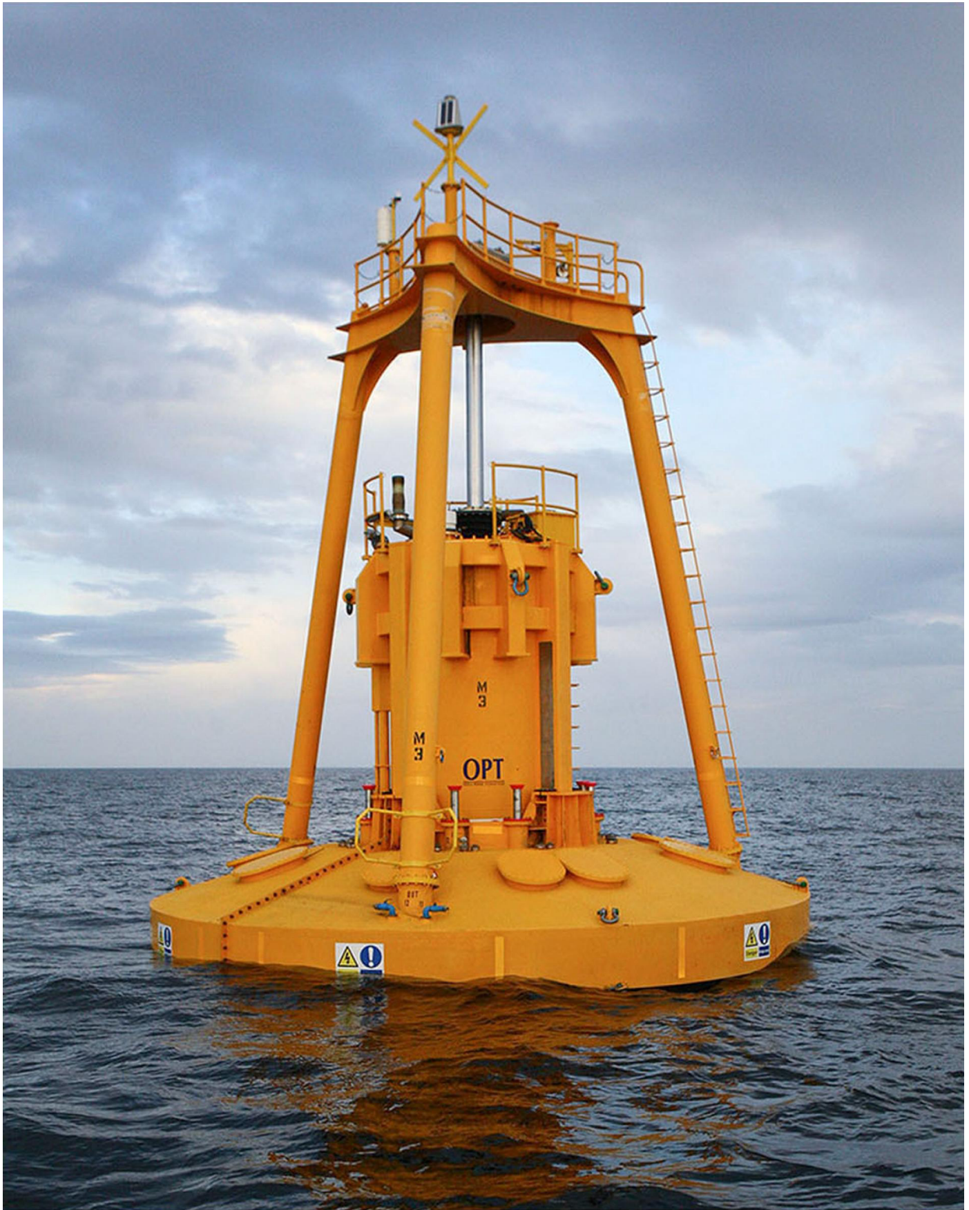
Specially designed buoys can use the rise and fall of ocean waves to generate energy.
