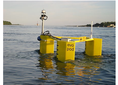
Evopod - A semi-submerged floating approach tested in Strangford Lough.
