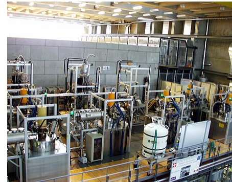
Set of hyperfrequency tubes (84 GHz and 118 GHz) for plasma heating by electron cyclotron waves on the Tokamak à Configuration Variable (TCV). Courtesy of SPC-EPFL.
