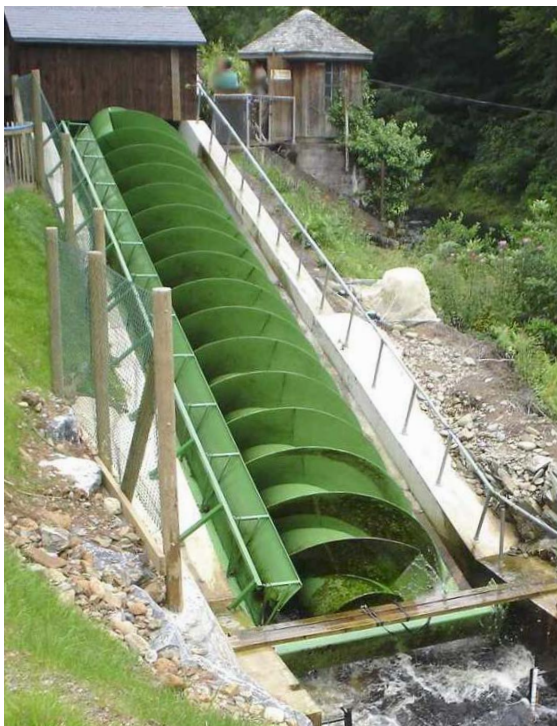
Figure 1-8. Archimedes screw for hydropower generation
