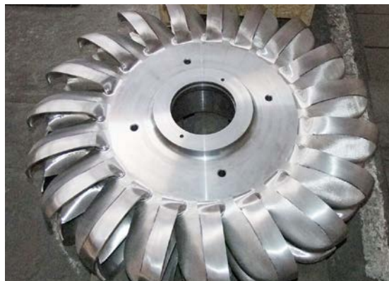
Figure 2-36. Examples of Francis, Pelton, and Kaplan turbines
