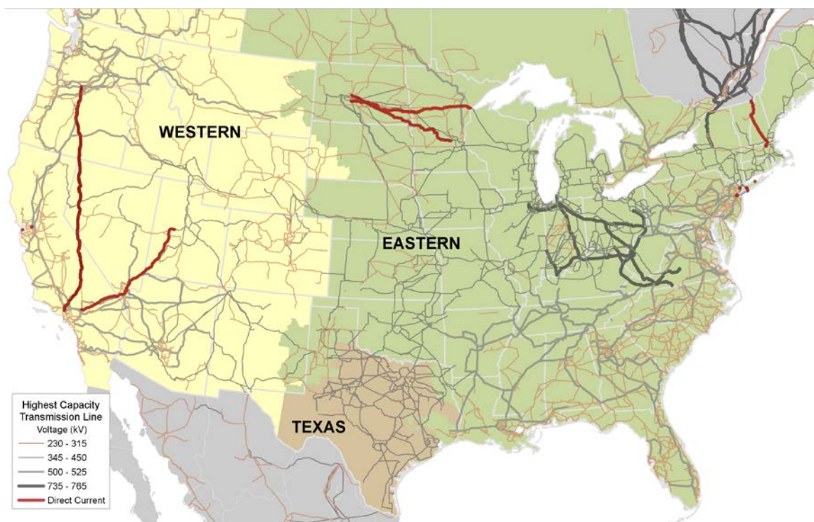
Figure 2-12. Transmission systems and three main grid interconnections in North America. In this map, the Quebec (Canada) Interconnection is part of the Eastern Interconnection.
