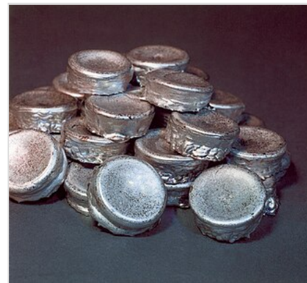
Enriched uranium produced at LLNL plant was collected as nuggets the size and thickness of several quarters.
