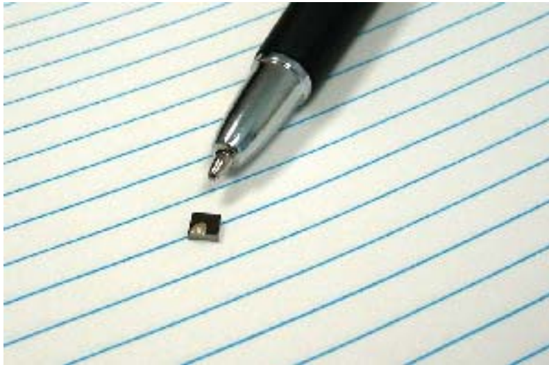
Figure 5-9 An MIS sensor for measuring acetylene gas levels in oil. The use of MIS gas-in-oil sensors can increase the number of transformers monitored due to their lower cost.
