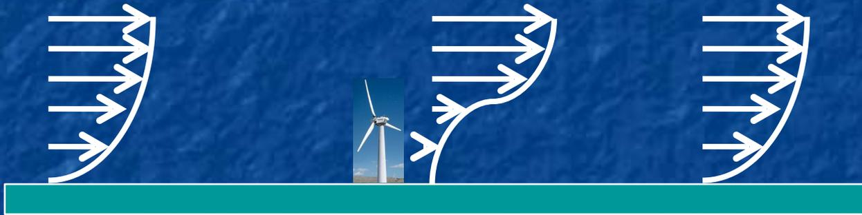
With turbines should be as tall/big as possible to capture higher speed upper winds:
