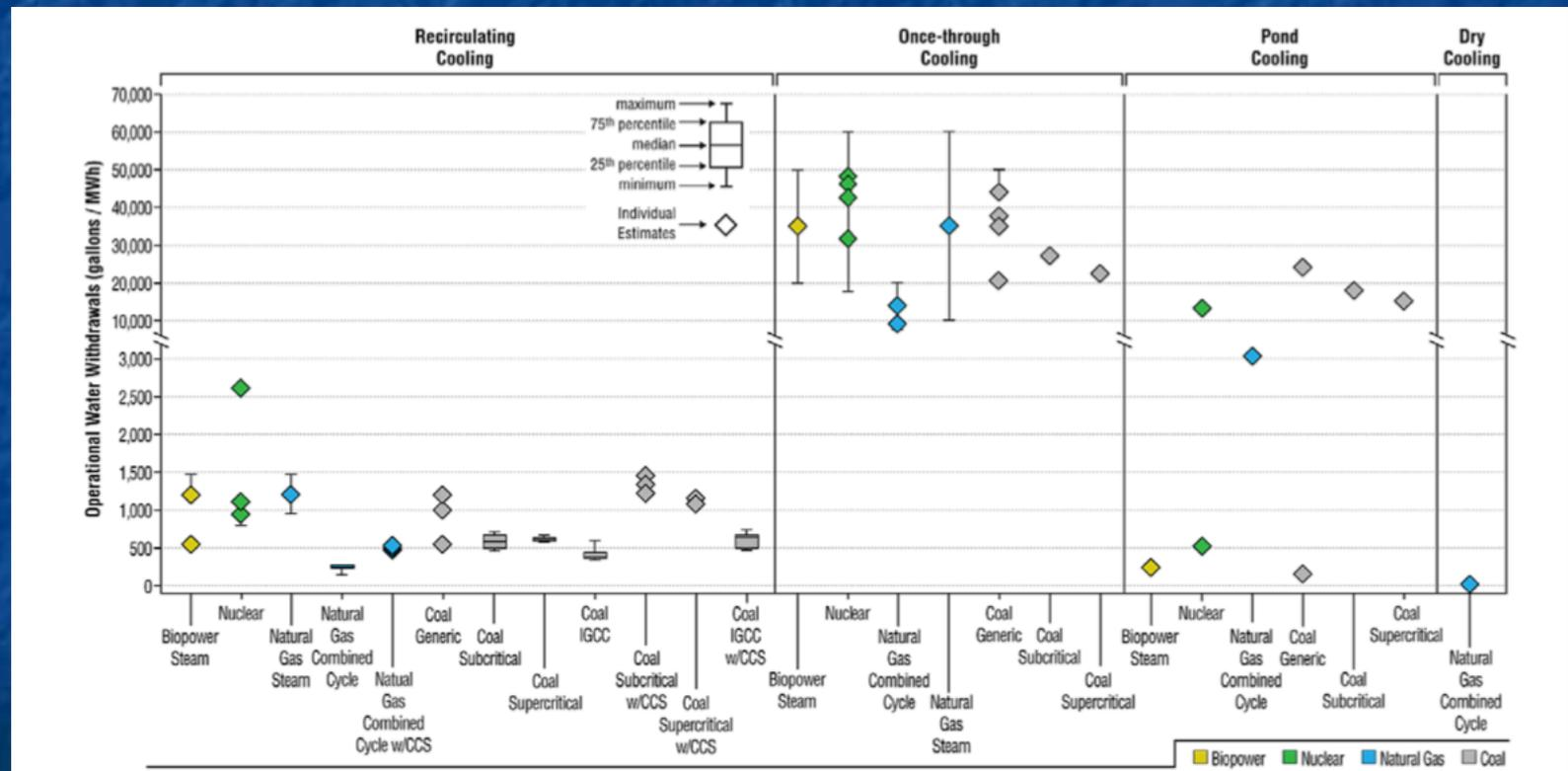
**Figure 2.** Operational water withdrawals for fuel-based electricity generating technologies. IGCC: integrated gasification combined cycle. CCS: carbon capture and storage.
