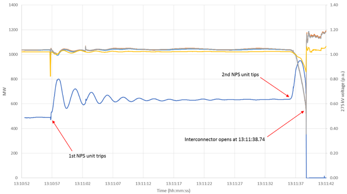
Figure 62 Heywood Interconnector MW flow, and SA system voltages for 2 December 1999 event
