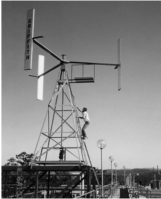
Figure 8: Three blade variable pitch VAWT developed by Kirke [25] clearly showing the counterweights incorporated in the blade pitch mechanism (photograph – copyright Brian Kirke).
