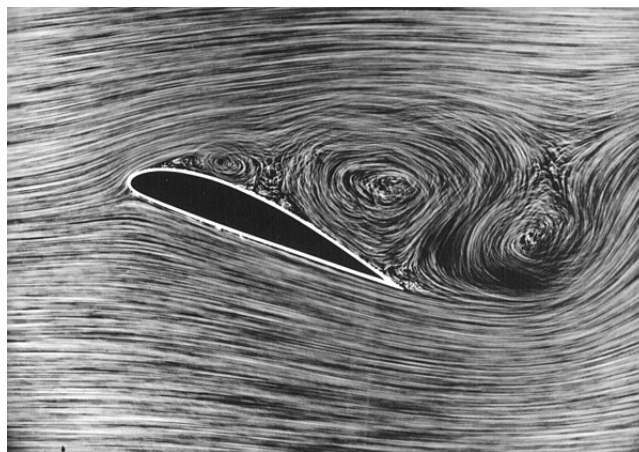
Airflow separating from a wing at a high angle of attack
