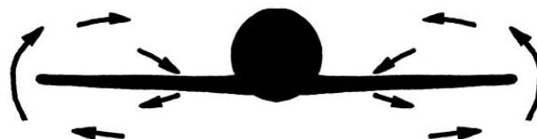
Cross-section of an airplane wing-body combination showing velocity vectors of the three-dimensional lifting flow
